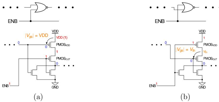
図 9: NOR RO in transistor level. (a) NBTI-sensitive RO. (b) NBTI-insensitive RO.
