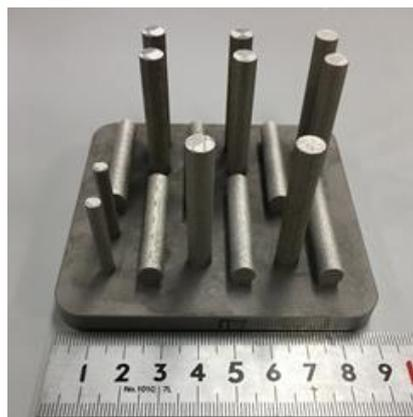
Fig. 2 Appearance of L-PBFed Zr-Nb-Sn alloy builds.
