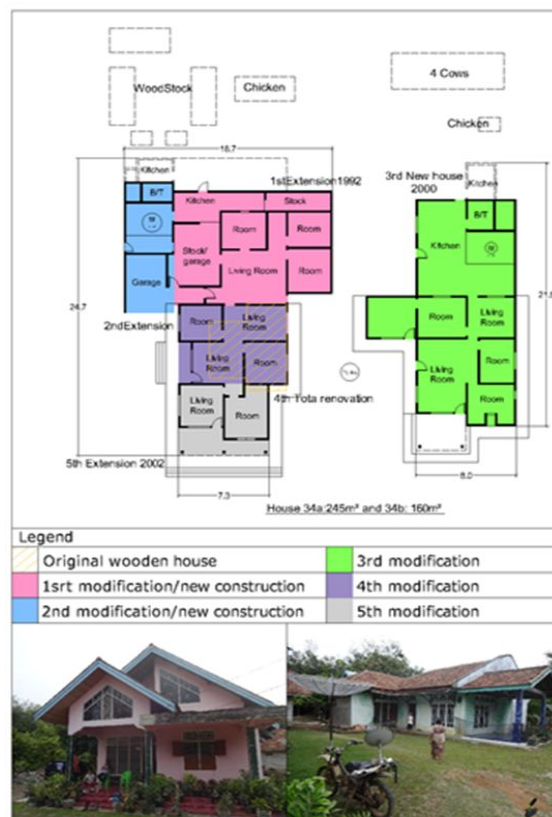
Fig. 2 Housing renovation in Sitiung
