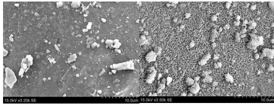
Fig. 4 (Left) The SEM-observed surface of the as-sampled hard scale and (Right) the rinsed surface.
