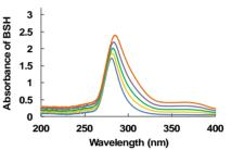
UV-visible Absorption Spectra of BSH/ND201 Complex
