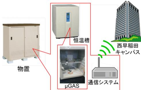
Fig.3 An early detection telemeter system of SO<sub>2</sub> and H<sub>2</sub>S in the ambient air at the southeastern of Mt. Fuji
