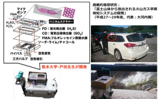
Fig.1 Survey of SO<sub>2</sub> and H<sub>2</sub>S in the ambient air by potable  $\mu$ Gas system in Owakudani, Hakone
