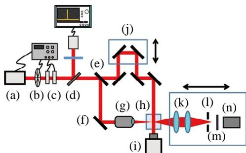
(a) fs-laser system, (b) optical chopper, (c) mechanical shutter, (d) half mirror, (e) beam splitter, (f) mirror, (g) objective lens, (h) cell, (i) camera, (j) optical pass delay, (k) objective lenses, (l) pin hole, (m) short-pass filter, (n) photomultiplier
