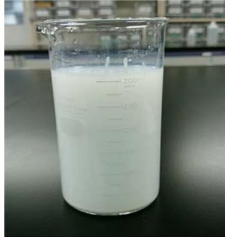
**Fig.3** (Water-TiO<sub>2</sub>) Nano-fluid
