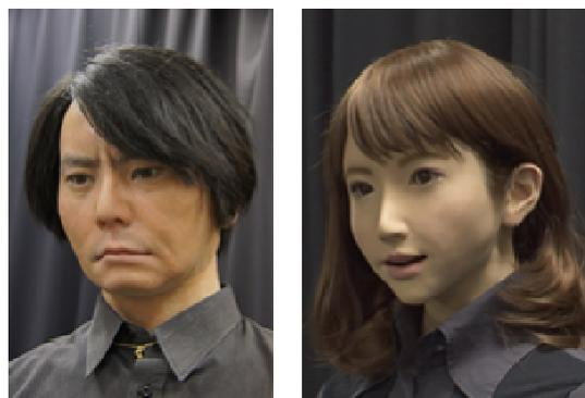
Fig. 1 Appearances of two android robots. (Left: HI2, Right: ERICA)
