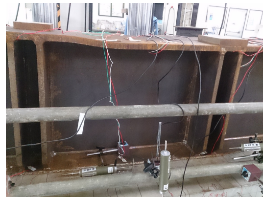
(b) Deformation of the top flange
