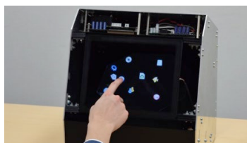
Figure 1 Aerial touch panel with haptic feedback
