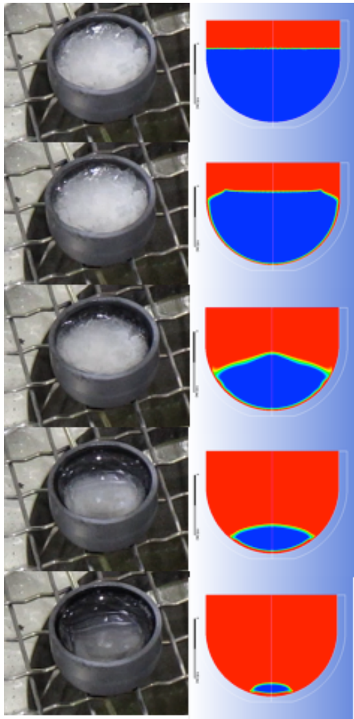
Fig. 5. Experimentally captured and numerically predicted melting front of the capsule at different instants
