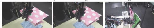
(d) Prediction of the folding failure. (e) Folding the target. (f) Inserting the target to the stand.
