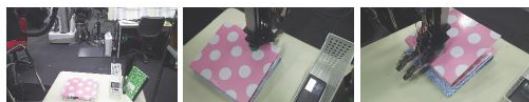
(a) Recognition of the environment. (b) After suction point refining. (c) Hand pose in suctioning.
