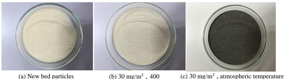
Fig. 4 Pictures of bed particle after experiments of PM collection.
