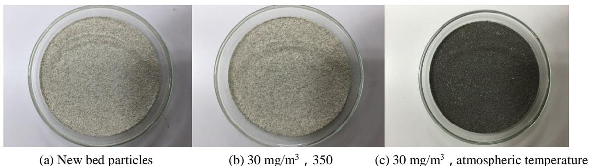
Fig. 5 Pictures of bed particle with K after experiments of PM collection.
