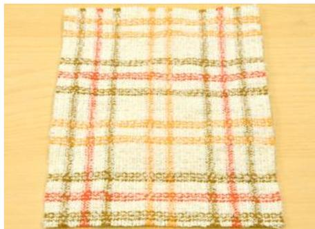
Fig. 2 Electric conductive fabric. (CS6001, Shibata Technotex)
