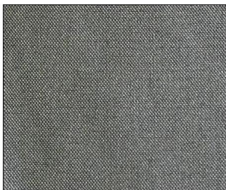
Fig. 4 Electric conductive fabric. (Osaka Electronics Industry)
