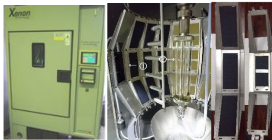
Fig.1 Xenon weather meter (left), internal sample holder (center) and exposure orientation (right)
