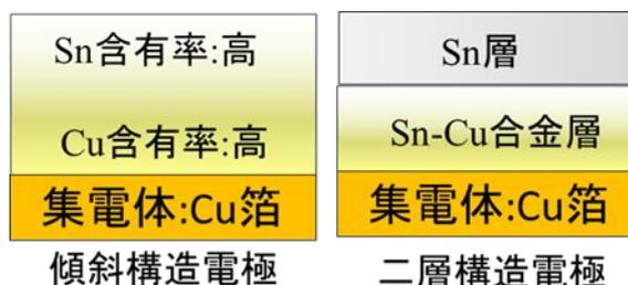
Fig. 5 Schematic model of Sn-Cu inclined/double layer electrode.
