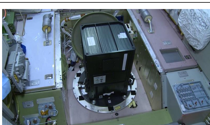
Figure 3: Mini-EUSO installed in the Zvezda module of the ISS. The velocity vector is usually toward bottom, in the side marked as '1' on Mini-EUSO.
