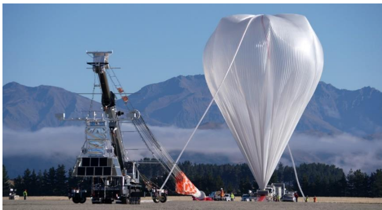
Figure 2: EUSO-SPB on the launch pad, in Wanaka. The payload is on the left, suspended from the crane which launched it.
