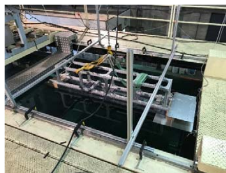
Fig. 2 Model ship on circulating water tank
