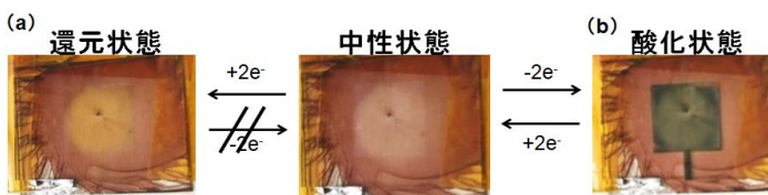
Fig.3 PQBT1 liquid crystalline thin film coated on ITO electrode at 85 °C. (a) electrochemical reduction, (b) electrochemical oxidation.
