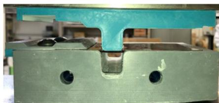
Fig.5 Press forming die made by 3D printer.
