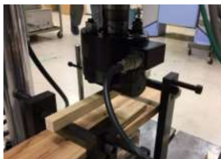
Fig. 2 Testing set-up for cyclic bending test.
