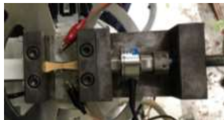
Fig. 1 Set up for XRD measurement.
