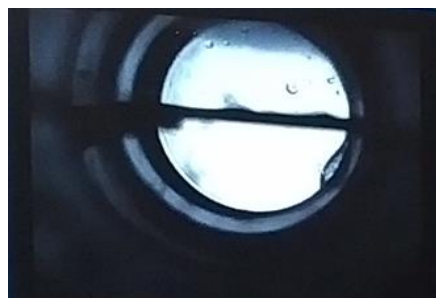
Fig. 4 The highly acidic interphase between scCO 2 and subH 2 O, observed by in-situ Raman spectroscopy.
