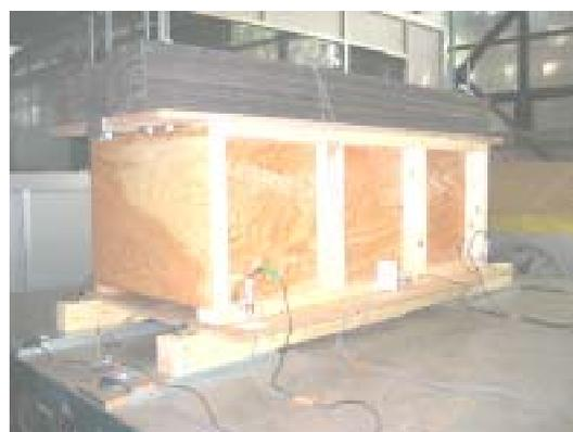
Fig.2. Shaking table test of a light frame construction model.
