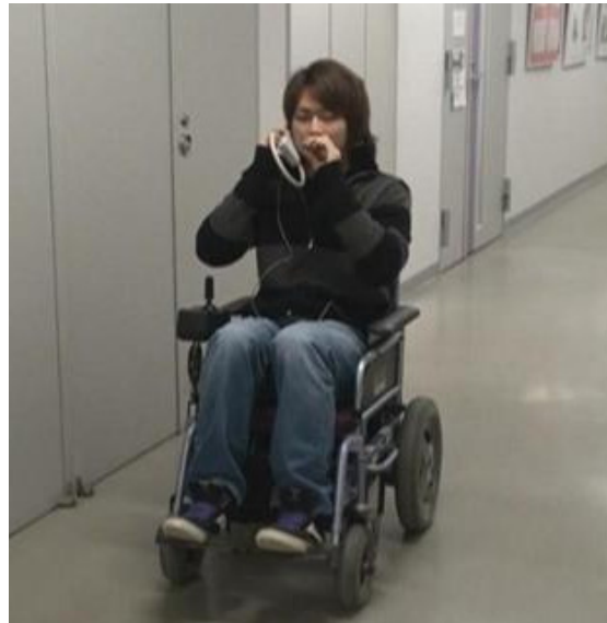
Fig. 3 : Trial operation of electrical powered wheelchair by using mouthpiece remote controller.
