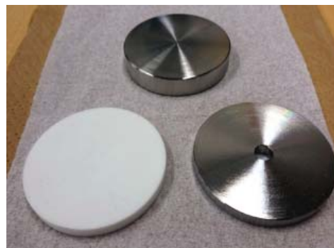
図3(上)SUS緩衝板:直径50mm・厚さ10mm (下左) \text{Al}_2\text{O}_3 円板:直径50mm・厚さ5mm (下右)SUS円板:〃・厚さ5mm・孔6mm
