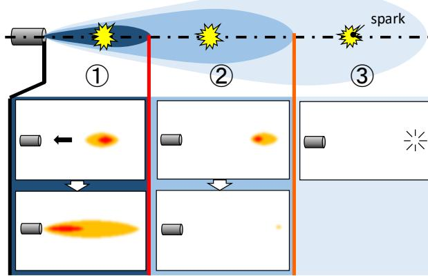
Fig. 2 Relationship between spark point and flame configuration.
