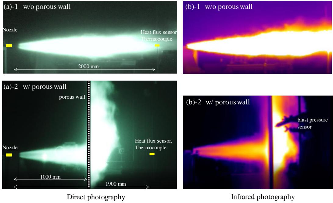
Fig. 4 Flame shape (a) without porous wall and (b) with porous wall ( $p_0 = 45$  MPa,  $\varphi = 0.8$  mm,  $x_w = 1000$  mm,  $x_i = 400$  mm).
