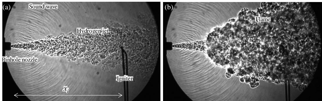
Fig. 3 Shadowgraph of hydrogen jet and diffusion flame near the pinhole nozzle ( $p_0 = 82 \text{ MPa}$ ,  $\varphi = 0.2 \text{ mm}$ ,  $x_{ig} = 250 \text{ mm}$ ).
