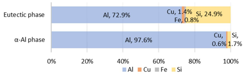
Fig. 3 Composition of α-Al and Eutectic phase in the samples applying EMS during solidification
