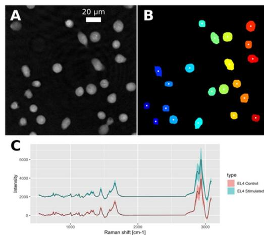
Figure 1: (A) Typical QPI image of EL4 T cells. (B) Automated segmentation of the objects in the field of view, where the center of each cells is used as an automatic target for the Raman laser excitation. (C) Typical average Raman spectrum of EL4 T cells with the standard deviation shown around the average (N=685).
