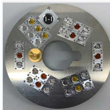
Fig. 3 Photograph of the samples mounted on the sample holder.
