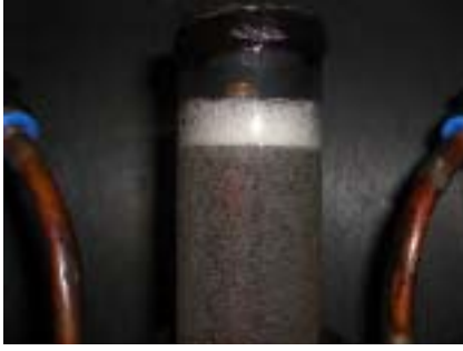
Fig.2 Micro-bubbles in the liquid fuel.
