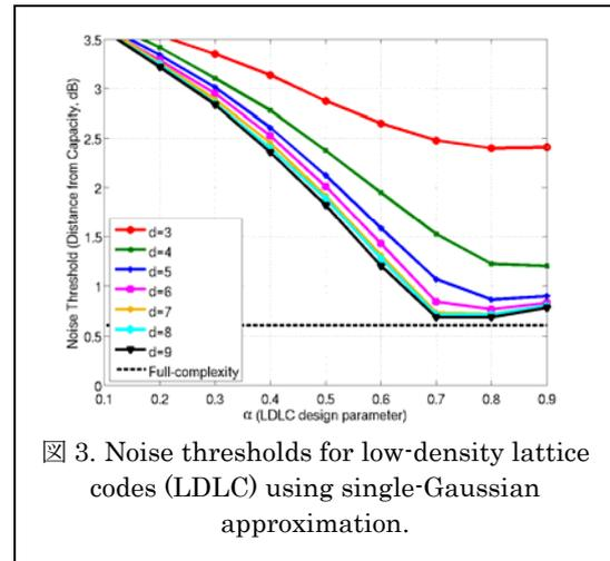
図3. Noise thresholds for low-density lattice codes (LDLC) using single-Gaussian approximation.
