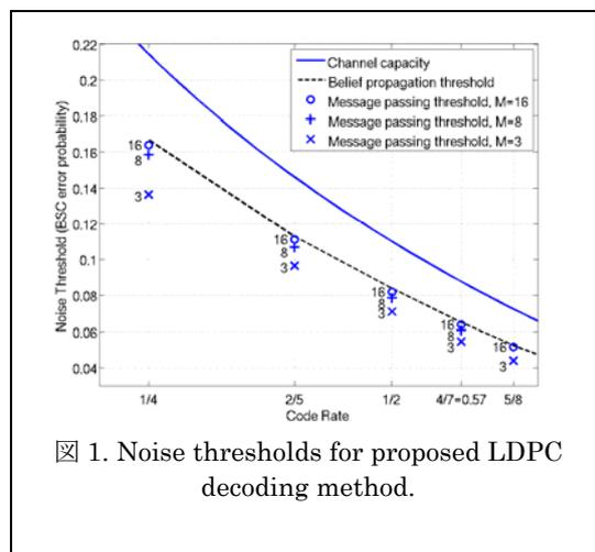
図 1. Noise thresholds for proposed LDPC decoding method.
