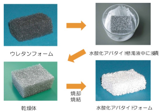
Fig. 1 Process of preparing a hydroxyapatite foam
