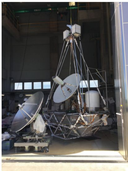
Figure 2: Photograph of the balloon-borne VLBI station during a hanging test in the assembly room in JAXA TARF. Sun shields and ballast boxes are not attached to the gondola at this time. The Taiki 1.5-m ground-based station is shown on the left.
