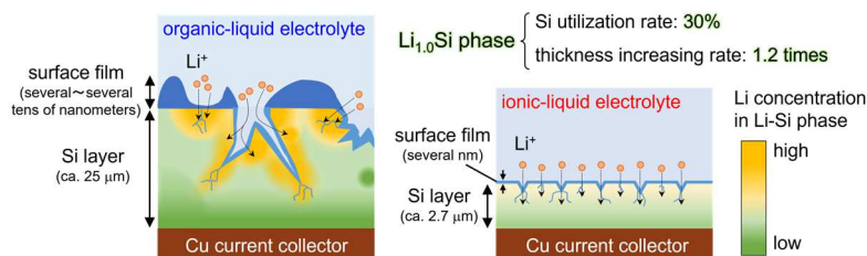
Fig. 3. Schematic illustration of Li-Si phase distribution in organic-liquid and ionic-liquid electrolytes.
