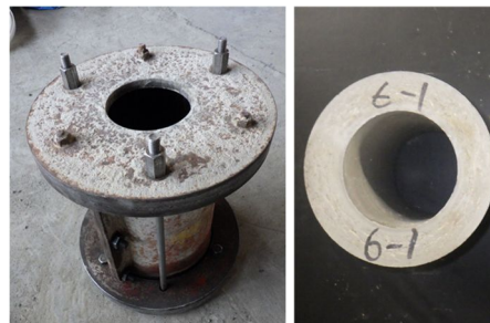
Fig.1 Concrete Formwork and Specimen
