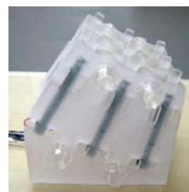
Fig. 2 Focused acoustic oscillator comprising nine (3 x 3) multilayer piezoelectric actuators (green rods).
