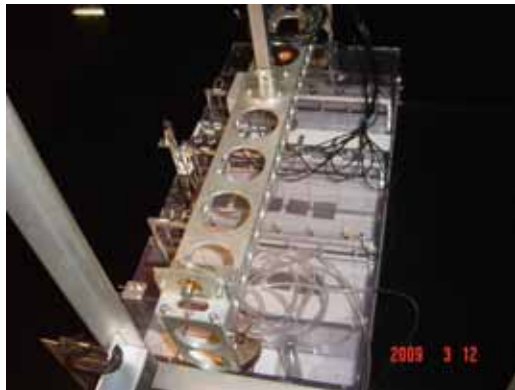
図1 供試船 (L=0.92m, B=0.45m, D=0.25m, d=0.10m, W=47kgf)
