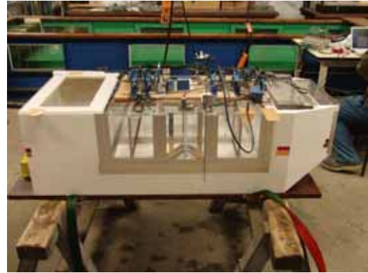
図2 供試船 (L=1.20m, B=0.50m, D=0.35m, d=0.175m, W=97kgf)
