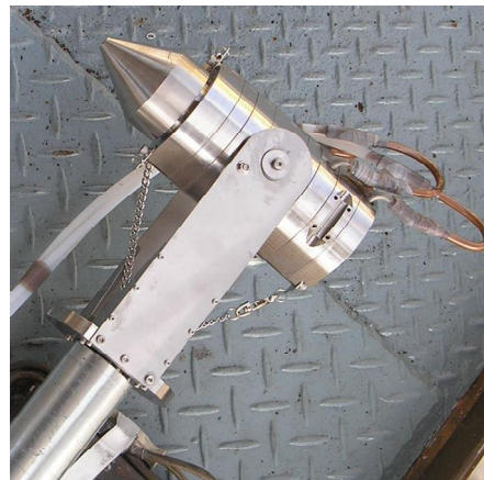
Fig.2 Picture of VIS impactor for \text{PM}_{10}/\text{PM}_{2.5} sampling in stack of stationary sources
