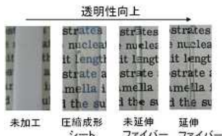
Figure 1 Changes in transparency of several processed materials of ‘crystalline’ fluorinated copolymers. (a) bulk PFA, (b) pressed-processing sheet, (c) crystalline fiber with drawn ratio = 3, (d) crystalline fiber with drawn ratio = 5.
