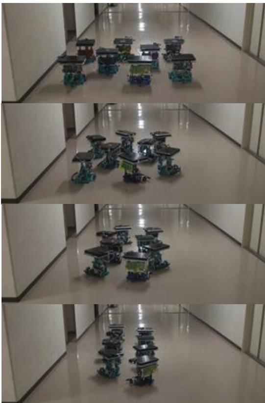
図 6 Snapshots of experiment of changing the width of the formation
