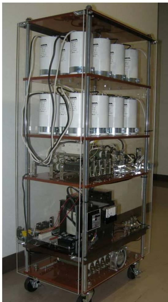
Figure 1, Picture of a constructed pulsed magnet. 1<sup>st</sup> stage: Charge resistor, 2<sup>nd</sup> stage: Transformer, Earth circuit, 3<sup>rd</sup> stage: Discharge, Trigger, and Crowbar circuit, 4, 5<sup>th</sup> stages: Capacitors (16 pieces)
