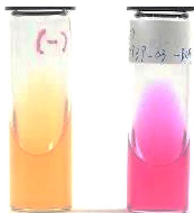
Fig. 2 The red coloration in the right sample shows the urease activity of the only strain that survived ammonia autotoxicity during the 2-week urea gel release.
