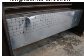
(a) 0.3_1.0 Photo 1 Deformed configuration in loading test
