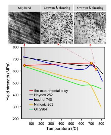
Fig.1 The yield strength as a function of the temperature of the developed Ni-Fe-based alloy and other Ni-based/Ni-Fe-based alloys. The predominant deformation behaviors in terms of dislocations interact with  $\gamma'$  precipitates at various temperatures.
