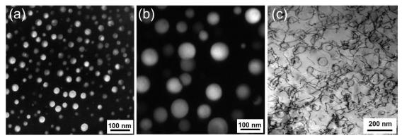
Fig.2 (a) and (b) TEM dark field images of  $\gamma'$  precipitate after heat treatment and creep test at 700°C 150MPa, respectively. (c) Creep deformation microstructure consists of Orowan loops around the  $\gamma'$  precipitates
