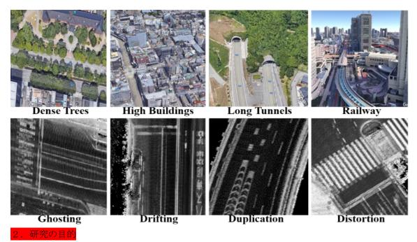
Accurate maps must be generated to control vehicles during the autonomous driving. The projected aimed to propose a mass-production framework to generate largescale <u>LIDAR</u> maps in size of cities and prefectures. Such a demand is challenging and unique in Japan as well as in the autonomous vehicle research field globally. Thus, the proposal investigated the following problems:
