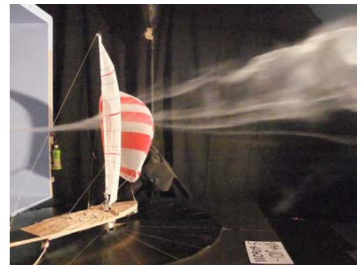
Fig.7 Comparison of stream line around sail between experiment and calculation (Top view, 120 degrees)
