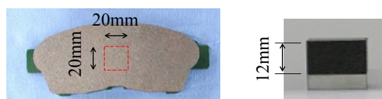
(a) Cutout position (b) Side view of test piece
