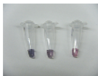
Fig. 5 Colorimetric detection of DNA-binding molecules in combination gold nanoparticles with PCR-based screening method; left, 0 nM DAPI, central, 100 nM DAPI, right, 1000 nM DAPI.
