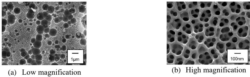
Fig. 2 Nanostructure on A5052 fabricated by anodizing & etching treatment.
